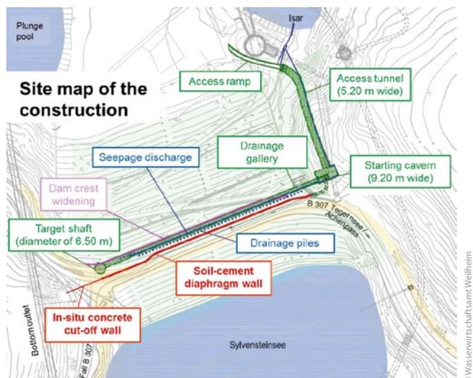
**Figure 1:** Sylvenstein reservoir: Site map of upgrade work on the Sylvenstein reservoir (diaphragm wall, drainage tunnel/inspection gallery, drainage piles)
